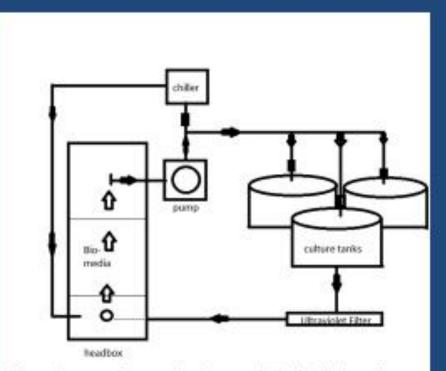
Culture tanks are currently set up and plumbing goes to the Ultraviolet filter located in a floor trench.
